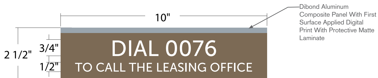
1 FRONT ELEVATION EE.01 Scale: 2" = 1'
