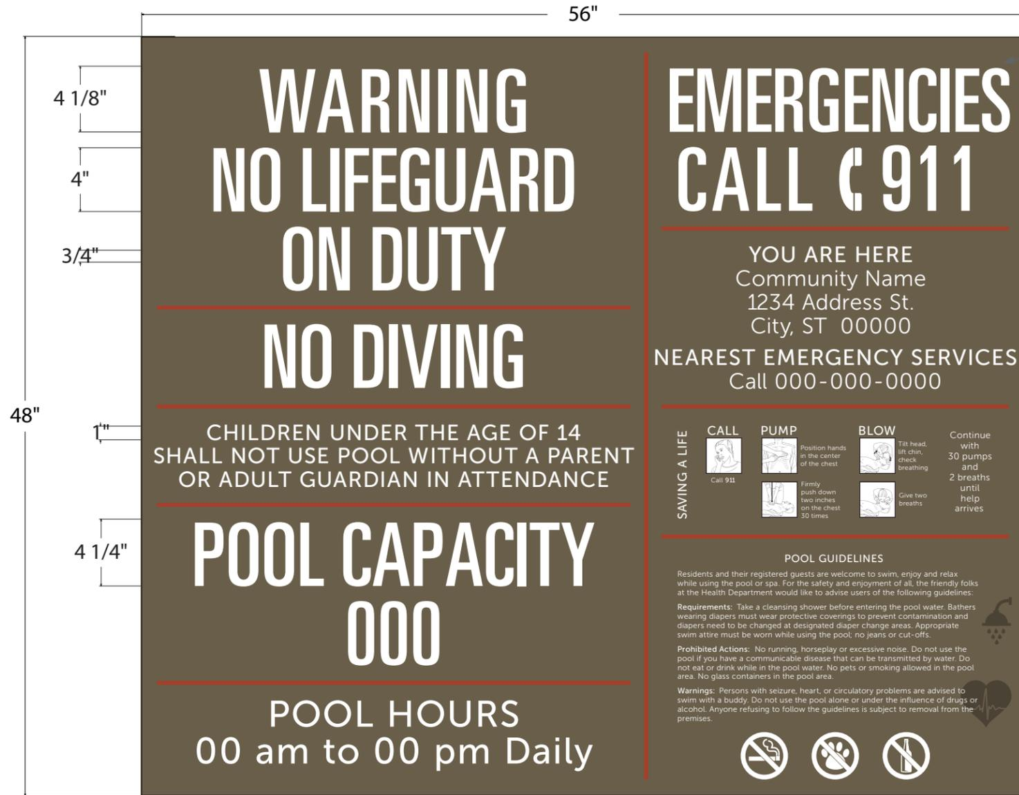
Dibond Aluminum Composite Panel With First Surface Applied Digital Print With Protective Matte Laminate
